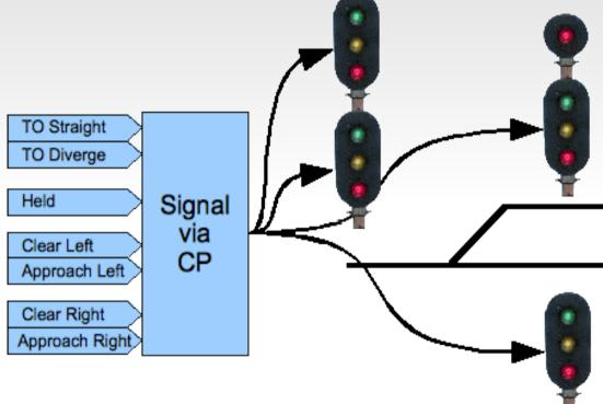
This method is similar to the signal aspect driver, but includes turnout control and possibly even occupancy detection on the same node. However it still requires an external controller or program such as JMRI to calculate the proper aspects. The original RR-CirKits LNCP is similar to this option.
