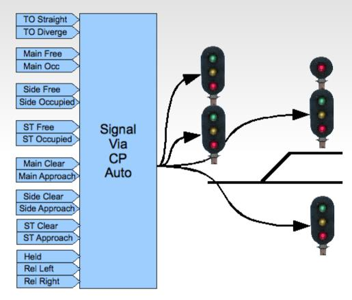
• It's also possible to build a signal controller that watches all related status Events from the railroad and CTC panel and makes independent decisions about the proper signal states and appearances. This type of controller would be able to control its signals without any external computer involvement.
