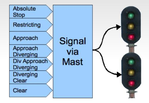
This method requires the minimum amount of command traffic to control the signals themselves. However it still requires an external controller or a program such as JMRI to monitor the layout and calculate the proper aspects. The Team Digital SHD2, Signalist SC1, and RR-CirKits SignalMan in NMRA Signal Aspect mode fall into this category.
