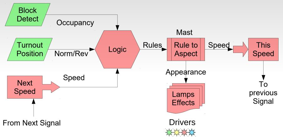
In typical existing systems the green items are part of the layout hardware, and the red items are taken care of by an attached computer.
