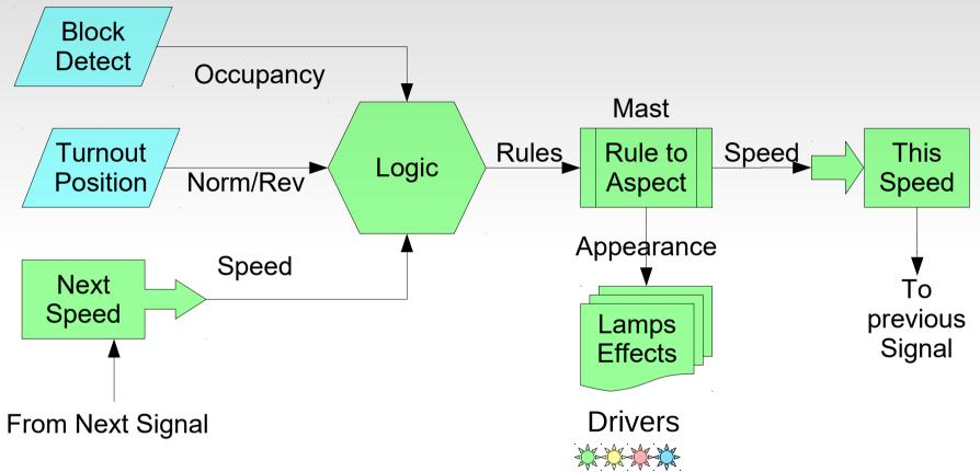
With the Signal LCC all of the control functions required for signaling exist locally. Light blue items are on a daughter card or different nodes.
