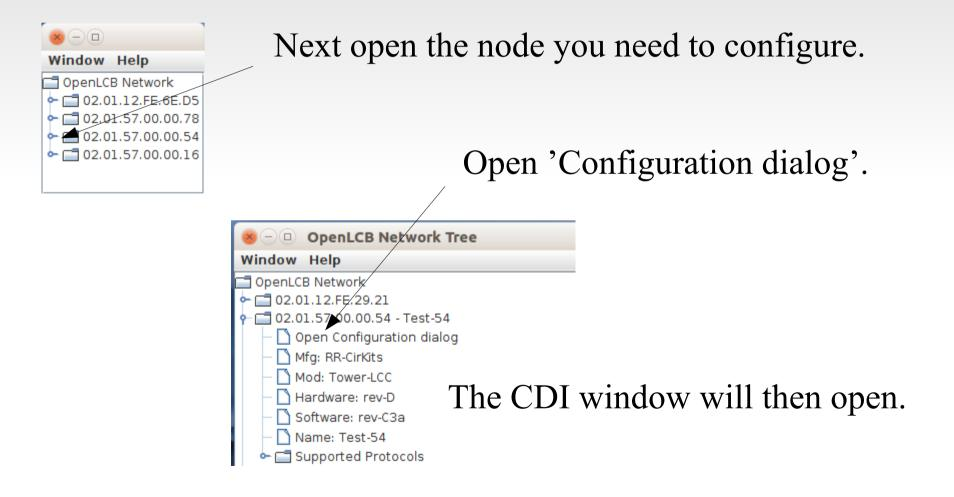
Because LCC is an open standard anyone can develop tools for it. One such developer is Robert Heller of Deepwoods Software. This is part of his model railroad software package. http://www.deepsoft.com/home/products/modelrailroadsystem/downloadmr/ Run the OpenLCB tool.
