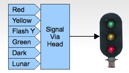
This method requires less command traffic than the previous one. However, if the controller does not know how to flash the signals, it may still result in constant streams of messages to be able to show flashing aspects. The Digitrax SE8c falls into this category. It normally only displays Green, Yellow, Red, and Dark. To show 'Flash Y' you need to alternate between sending Yellow and sending Dark. Got Lunar?
