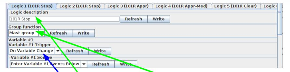
Enter the logic description and set the function to Mast Group. Logic defaults to watching variable changes.
