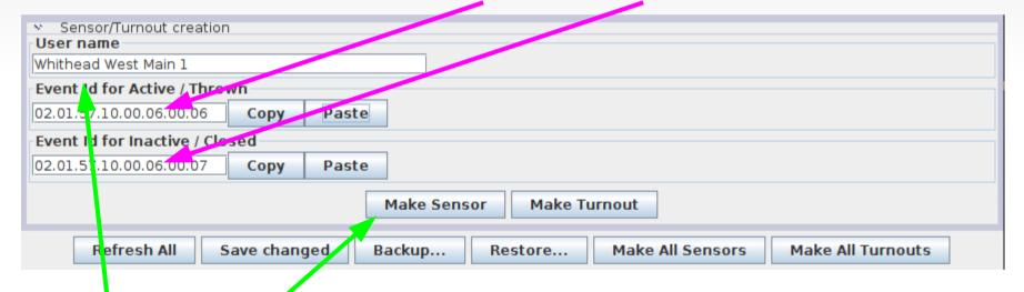
Enter the JMRI user name for this sensor, (or turnout) then click on the Make Sensor button. This item will automatically be added to your JMRI Sensor (or turnout) table. Be sure to save the table for future use. Normally this data will become part of a 'Panels' file, and be synchronized with the node when loaded.
