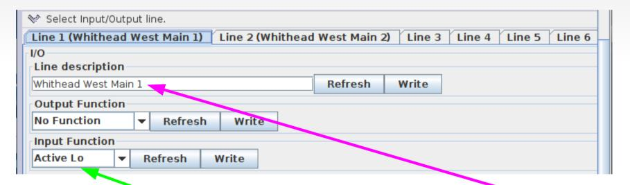
Lets start by connecting a block sensor to an input. Its description is 'Whithead West Main 1' so we enter it in the description block and 'Write' it to the node. Detectors are Input Functions with 'Active Lo' so we set that and write it. For a normal Input be sure that the Output Function is set to 'No Function'. Of course 'Line 1' is the one connected to our first block detector.
