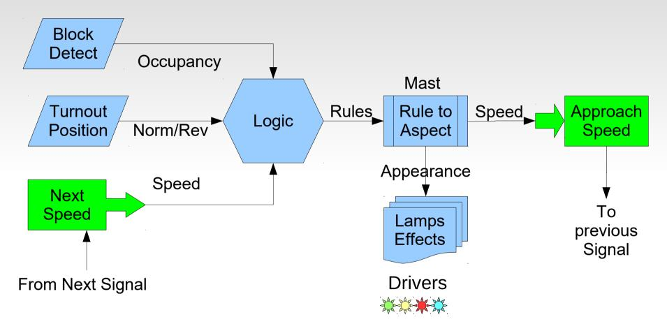
Paste the next masts 'Up Link EventID' from the mast to a local track circuit. This creates a virtual link directly into the logic variables by virtual name rather than by using actual event numbers. The logic for a mast can be setup, or mass produced, without knowing any actual mast IDs ahead of time.
