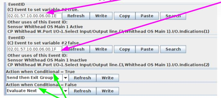
• These default actions are normal for mast logic conditionals. If the condition is true, then any actions are sent, and all less restrictive aspects are skipped.
