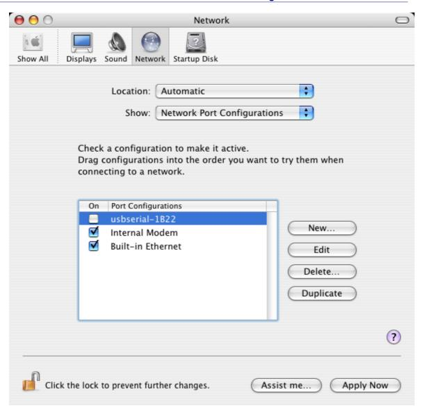
At this point, it is possible to exit Network and use the device as a COM port. If you wish to set the device up a a modem for an Internet connection, select the new port from the Show list to display the window below. Please note that the FT2232C device has two ports available and these must be configured separately.
