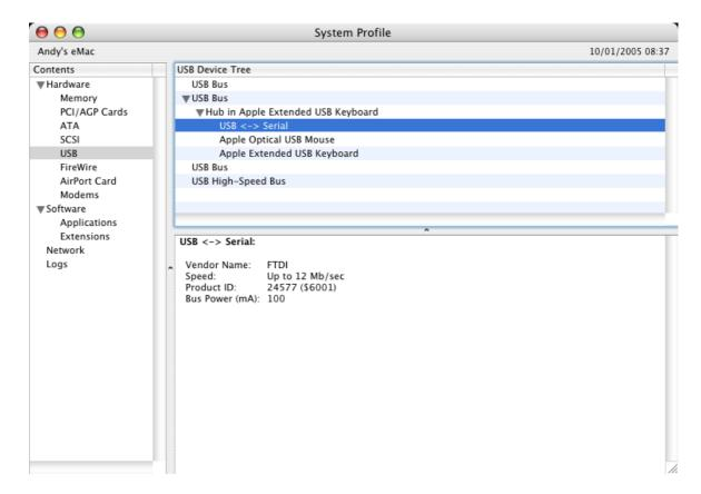
If the device does not work after installing the driver, it is likely to be because the PID is not supported by the driver. If this is the case, contact FTDI Support with the PID that needs to be added to the driver. If the VID is not 0x0403, it is likely that the device is not an FTDI device and we cannot support it.
