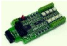
**Remote Sensing** The BOD-8 uses small CT (Current Transformer) detection coils placed directly on the track feeders between the rail and the power bus. Lengths of Cat-5 cable are the usual way to connect the coils to the detector boards. CT coil sensors cause no track voltage losses like those associated with diode drop detectors.
