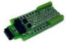
**OIB-8** (Opto Isolator Board - 8 input) This 8 input board is used when a non-isolated source of voltage needs to be monitored and input to the LNCP. One example would be to monitor the DCC voltage on a set of points to determine the position of a turnout without using auxiliary contacts. Another example would be the detection of trains on a three rail or overhead wired layout using isolated rail sections.
