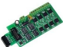
**SCSD-8** (Single Coil Solenoid Driver) The SCSD-8 Output Module is designed to drive individual solenoid coils or other high voltage high power devices. Normally the input voltage should not exceed 35VDC. The SCSD-8 board is optically isolated from the driving circuitry to protect the LNCP or other control device from the high power outputs.
