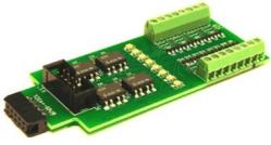
This 8 input board is used when a non-isolated source of voltage needs to be monitored and input to the Signal LCC-32H. One example would be to monitor the DCC voltage on a set of points to determine the position of a turnout without using auxiliary contacts.
