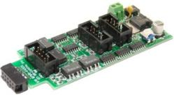
The SMD-8 board contains 8 individual, optically isolated, H-Bridge drivers. This allows the board to be powered from any supply between 9 Volts and 27 Volts. It is primarily designed to drive stall motor turnout machines such as those found in Tortoise® and Switchcraft® machines. It is also suitable for the higher current required by the MTB-MP1 and MTB-MP5 machines.
