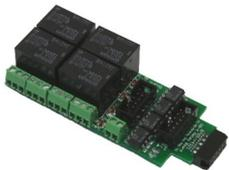
Relay Board - 4 is a Quad 10A SPDT relay board with logic level drivers. It is suitable for use with Signal LCC-32H or other logic level output devices. It requires 12V auxiliary power to drive the relay coils. Auxiliary power is optically isolated from the logic inputs for double isolation. LED indicators for each relay make it easy to monitor activity.
