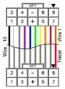
Note: I/O line 1 is wire 10, I/O line 8 is wire 1. 10 position IDC connector
