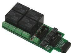
Relay Board - 4 is a Quad 10A SPDT relay board with logic level drivers. It is suitable for use with Tower LCC or other logic level output devices. It requires 12V auxiliary power to drive the relay coils. Auxiliary power is optically isolated from the logic inputs for double isolation. LED indicators for each relay make it easy to monitor activity.
