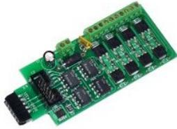
The SCSD-8 Output Module is designed to drive individual solenoid coils or other high voltage high power devices. Normally the input voltage should not exceed 27VDC. The SCSD-8 board is optically isolated from the driving circuitry to protect the Tower LCC or other control device from the high power outputs. When driving single coils or high power loads configure the line as a steady output.
