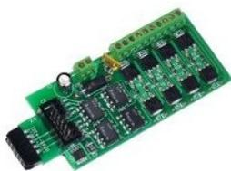
The SCSD-8 Output Module is designed to drive individual solenoid coils or other high voltage high power devices. Normally the input voltage should not exceed 35VDC. The SCSD-8 board is optically isolated from the driving circuitry to protect the WatchMan or other control device from the high power outputs. When driving single coils or high power loads configure the 'Type' as 'Driver'.
