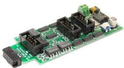
The SMD-8 board contains 8 individual, optically isolated, H-Bridge drivers. This allows the board to be powered from any supply between 9 Volts and 18 Volts. It is primarily designed to drive stall motor turnout machines such as those found in Tortoise® and Switchcraft® machines. Do not exceed 15VAC or 24VDC at the power input.
