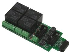
Relay Board - 4 is a Quad 10A SPDT relay board with logic level drivers. It is suitable for use with WatchMan, TC-64, LNCP, or other logic output devices. It requires 12V auxiliary power to drive the relay coils. Auxiliary power is optically isolated from the logic inputs for double isolation. LED indicators for each relay make it easy to monitor activity.
