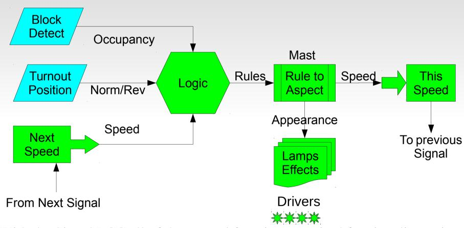
With the Signal LCC all of the control functions required for signaling exist locally. Light blue items are a daughter card or different nodes.
