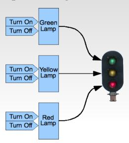
This is a powerful but complicated approach. It requires that the controller individually turn each lamp on or off. This can cause excessive control traffic and latency causes poor timing of flashing signals. There is also a cost/complexity trade off where lower cost drivers (more outputs per board) requires more wiring. Typically simple drivers lack special effects like fading and flashing.
