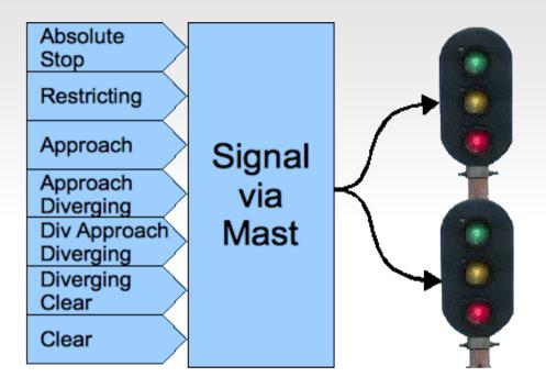
This method requires the minimum amount of command traffic to control the signals themselves. However it still requires an external controller or a program such as JMRI to monitor the layout and calculate the proper aspects. The Team Digital SHD2, Signalist SC1, and our RR-CirKits SignalMan in NMRA Signal Aspect mode fall into this category.
