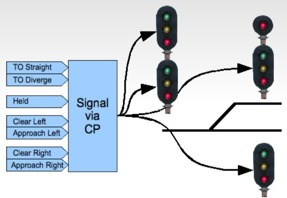
This method is similar to the signal aspect driver, but includes turnout control and possibly even occupancy detection on the same node. However it still requires an external controller or program such as JMRI to calculate the proper aspects. The original RR-CirKits LNCP is similar to this option.
