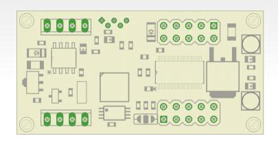
Lower cost and smaller board. (25mm x 50mm)
