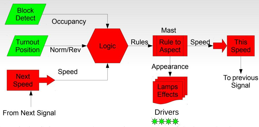
In typical existing systems the green items are part of the layout hardware, and the red items are taken care of by an attached computer.
