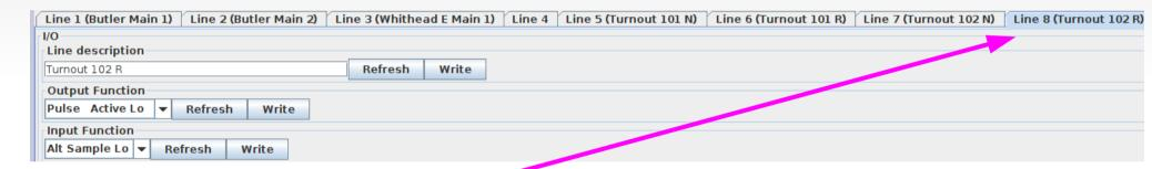
We use the input for Line 8 and connect it to a push button. We set the 'Input Function' to be 'Alt Sample Lo'. This means that each time the input goes low it will alternate the function state. The line still sends its output to drive the turnout as before. We can also use the same line (physical wire) as an input by sampling it.
