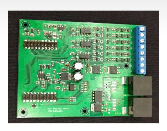
8-channel Block occupancy detector Adjustable sensitivity Feedback via LCC Circuit breaker Adjustable current limit Turn off staging track Railcom to determine which train is on the track Loco CV readout POM Staggered block power turn-on Auto reverse channel
