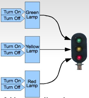
This is a powerful but complicated approach. It requires that the controller individually turn each lamp on or off. This can cause excessive control traffic and latency causes poor timing of flashing signals. This is the method used by CMRI.
