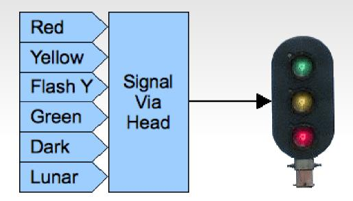
This method requires less command traffic than the previous one. However, if the controller does not know how to flash the signals, it may still result in constant streams of messages to be able to show flashing aspects. The Digitrax SE8c falls into this category. It normally only displays Green, Yellow, Red, and Dark. To show 'Flash Y' you need to alternate between sending Yellow and sending Dark. Got Lunar? Nope!
