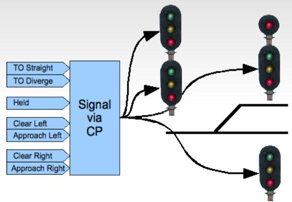
This method is similar to the signal aspect driver, but includes turnout control and possibly even occupancy detection on the same node. However it still requires an external controller or program such as JMRI to calculate the proper aspects. The old RR-CirKits LNCP is similar to this option.
