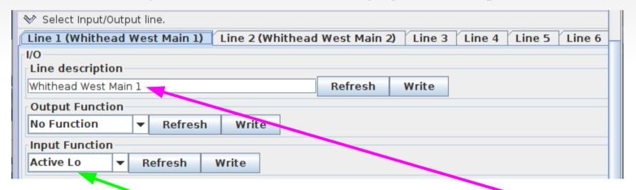
Lets start by connecting a block sensor to an input. Its description is 'Whithead West Main 1' so we enter it in the description block and 'Write' it to the node. Detectors are Input Functions with 'Active Lo' so we set that and write it. For a normal Input be sure that the Output Function is set to 'No Function'. Of course 'Line 1' is the one connected to our first block detector.
