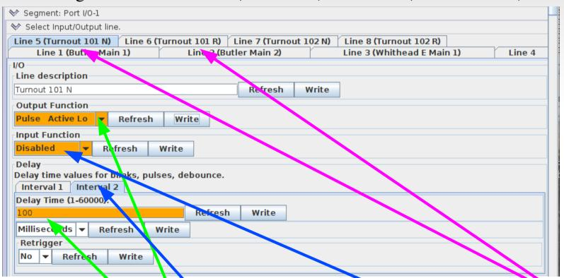
Our turnouts are controlled by Kato dual coil solenoids. This requires dual line drivers and 100mS pulse outputs. Normally inputs are disabled for Output Functions. Note: Use Interval 2 for pulse length. Interval 1 is the pulse delay.
