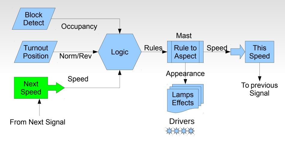
Paste the next masts 'Up Link EventID' from any mast to a track circuit. This creates a virtual link directly into the logic variables by virtual name rather than by using actual event numbers. The logic for a mast can be setup, or mass produced, without knowing any actual mast IDs ahead of time.
