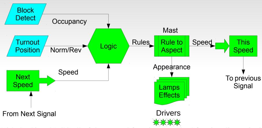
With the Signal LCC all of the control functions required for signaling exist in a single node. Light blue items are taken care of with a daughter card.
