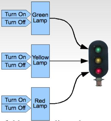
This is a powerful but complicated approach. It requires that the controller individually turn each lamp on or off. This can cause excessive control traffic and potentially poor timing of flashing signals. This is the method used by CMRI and currently (as of June 2017) available LCC equipment.
