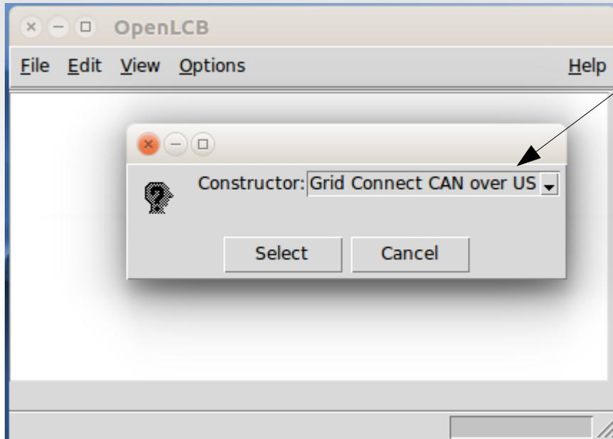
If you are using the LCC Buffer-USB as your interface device, then select 'Grid Connect CAN over USB'.
