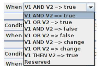
A statement may optionally send an event when true. To send an event define the event to be sent and check the 'Enable' check box. Events sent may be LocoNet sensor, switch, or switch feedback messages. Events may also be NMRA DCC Signal Mast commands. (mast number plus aspect)
