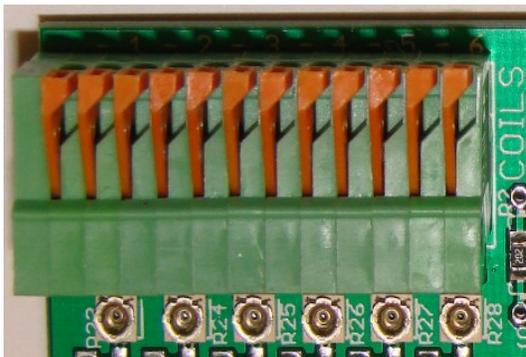
The opposite end of each CAT5 pair is connected to the compression connector labeled 'COILS' shown here. Strip the insulation from the wires for about 1/4”-3/8” before inserting them into the connector. Each of the six pairs connects to its own two compression points, numbered from left to right. (-1 -2 -3 -4 -5 -6) To make it easier to insert the wires or remove them simply press the orange quick release tabs toward the center of the connector using your finger nail or a small screwdriver.
