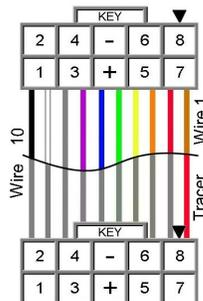
Note: I/O line 1 is wire #10, I/O line 8 is wire #1. 10 position IDC connector
