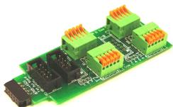
**FOB-8** (Fan Out Board) This board is a convenient way to convert from the LNCP 10 pin ribbon cable signal outputs to compression terminals at the signal masts themselves. The manually operated quick release connectors will accept wire sizes down to the small #36 AWG magnet wire found in some signals.
