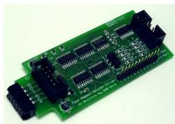
This output board drives up to 4 four aspect signal heads with 9VDC. The outputs are multiplexed to allow 4 heads on a single 10 wire flat ribbon cable. LED current dropping resistors are included on the board allowing the signals to be directly attached to the cables without purchasing any extra hardware for each signal. To control the fourth aspect two CV's are required and
