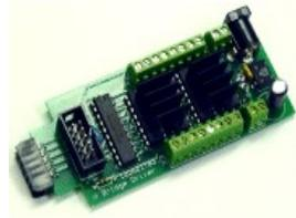
The DCDB-8 drivers include clamp diodes and may be used to directly drive inductive loads such as relay or solenoid coils if desired. The outputs are wired in an "H" bridge configuration but may be used single ended. Both positive and negative common return points are provided for single ended operation.
