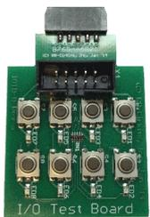
This board is a convenient way to test a port. It may be used for testing inputs or outputs, and includes 8 LEDs and 8 push buttons. The LEDs light when each output is low. The push buttons pull the inputs low. Both male and female I/O connectors make it easy to add in series with another cable.
