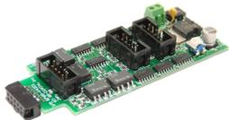
The SMD-8 board contains 8 individual, optically isolated, H-Bridge drivers. This allows the board to be powered from any supply between 9 Volts and 18 Volts. It is primarily designed to drive stall motor turnout machines such as those found in Tortoise® and Switchcraft® machines. Do not exceed 15VAC or 24VDC at the power input.
