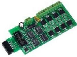
The SCSD-8 Output Module is designed to drive individual solenoid coils or other high voltage high power devices. Normally the input voltage should not exceed 35VDC. The SCSD-8 board is optically isolated from the driving circuitry to protect the Tower Controller Mark II or other control device from the high power outputs. When driving single coils or high power loads configure the 'Type' as 'Driver'.
