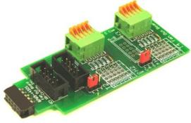
This board is a convenient way to convert from 10 pin ribbon cable to compression terminals. It may be used for inputs or outputs, and includes pads for mounting resistors such as required for connecting LEDs used for direct drive signals or panels.
