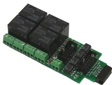
Relay Board - 4 is a Quad 10A SPDT relay board with logic level drivers. It is suitable for use with Tower Controller Mark II, TC-64, LNCP, or other logic output devices. It requires 12V auxiliary power to drive the relay coils. Auxiliary power is optically isolated from the logic inputs for double isolation. LED indicators for each relay make it easy to monitor activity.
