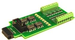
This 8 input board is used when a non-isolated source of voltage needs to be monitored and input to the Tower Controller Mark II. One example would be to monitor the DCC voltage on a set of points to determine the position of a turnout without using auxiliary contacts.
