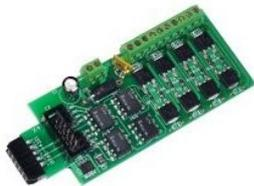
The SCSD-8 Output Module is designed to drive individual solenoid coils or other high voltage high power devices. Normally the input voltage should not exceed 35VDC. The SCSD-8 board is optically isolated from the driving circuitry to protect the TowerMan or other control device from the high power outputs. When driving single coils or high power loads configure the 'Type' as 'Driver'.
